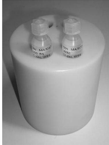
**Figure 1.** IRSN thyroid phantom for intercomparison (left), SCK•CEN thyroid phantom for calibration (right).
