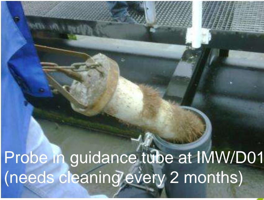
Probe in guidance tube at IMW/D01
